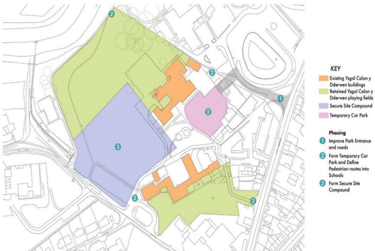
Figure 31: Construction sequencing and operation of the school
